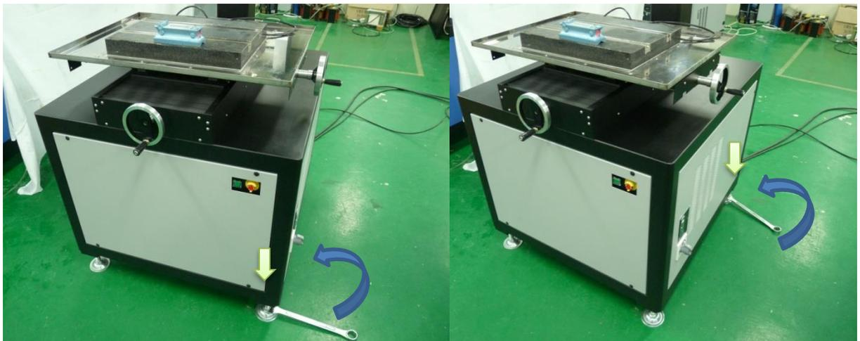
3. Turn the leveling bolt on the machine's right side counterclockwise to lower the right side.
