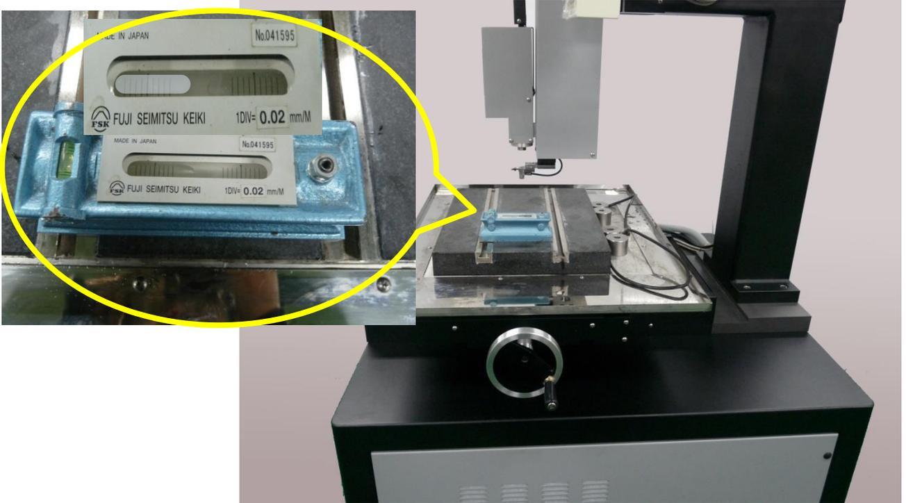
1. Place the level in the Y-axis direction.
