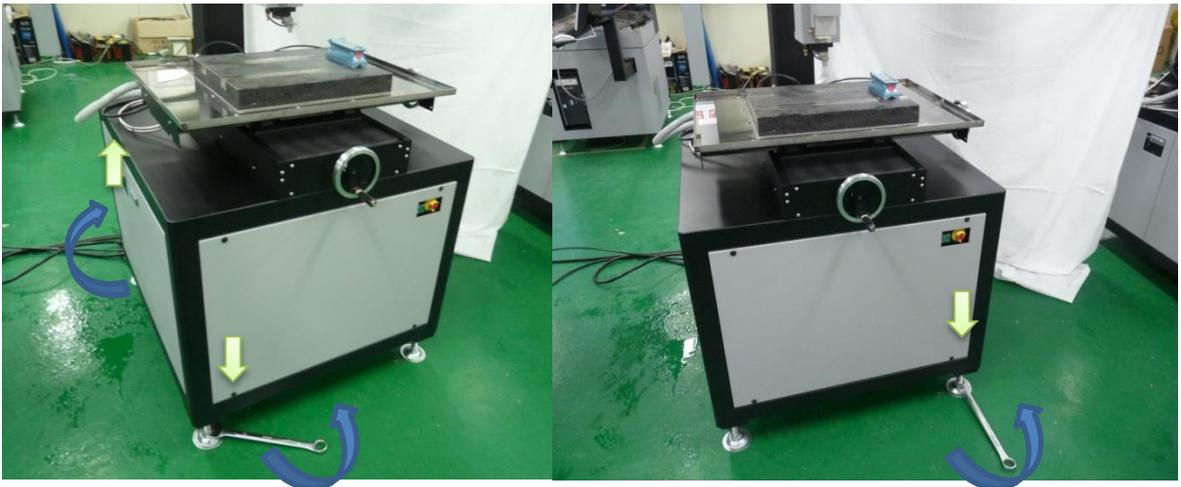
3. Turn the leveling bolt on the machine's front side counterclockwise to lower the front part.
