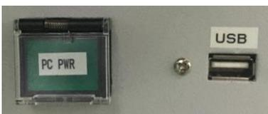
⑥ Turn on the power of the machine by pressing the POWER switch in the front panel of the computer.
