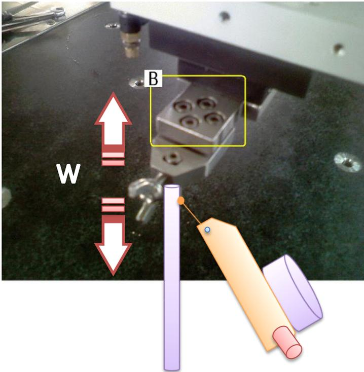
Use the bolts in the "B" area to correct the vertical.
