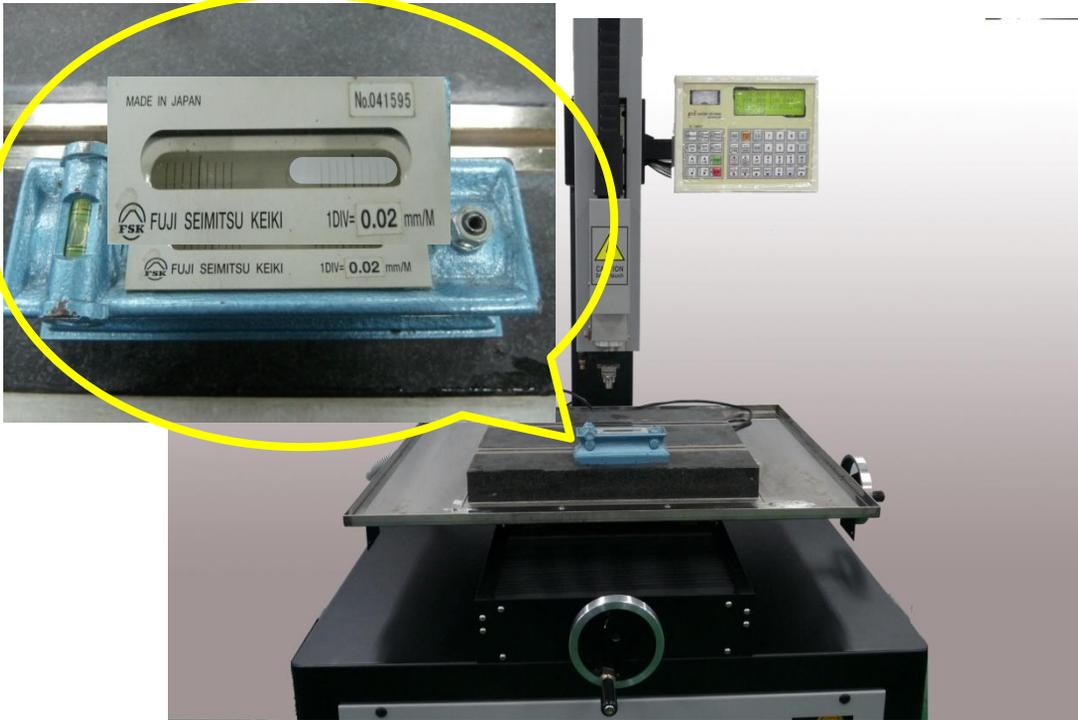
1. Place the level in the X-axis direction.
