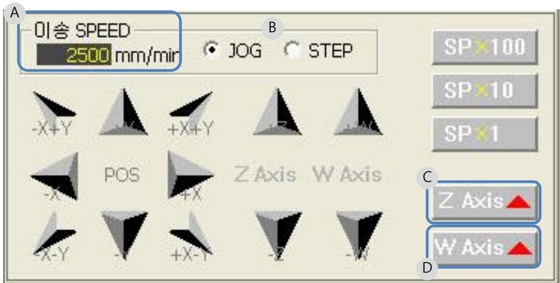
Controls the feed of each axis.
